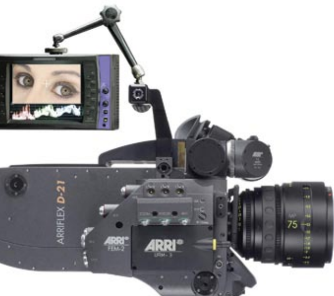
The Functional Expansion Module FEM-2 contains motor drivers for lens motors, hardware and software for the Lens Data System as well as a slot for an optional radio. With the Universal Radio Module URM-3 installed, the D-21 and its lens can be easily and quickly controlled by the ARRI Wireless Remote System (WRS)
