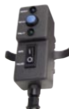
The SFR-1 can start (REC) and pause (PAUSE) recording of the SONY HDCAM SR field recorder. In addition it can play back a few seconds of the last take (REVW) and shows when the deck is recording (green TALLY LED) or ready to record (blue READY LED)
